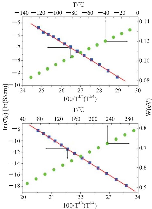
Fig. 2. Temperature dependence of dc conductivity  $\sigma_{dc}$  (solid squares, bottom and left axes) and the hopping energies  $W$  (solid circles, top and right axes) for CCTO ceramics in (a) low temperature range and (b) high temperature range
