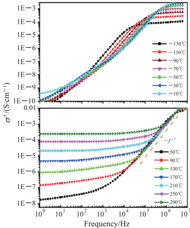
Fig. 1. Frequency dependence of conductivity  $\sigma'$  of CCTO in two temperature ranges: (a)  $-130^\circ\text{C}$  to  $10^\circ\text{C}$ ; (b)  $50^\circ\text{C}$  to  $290^\circ\text{C}$
