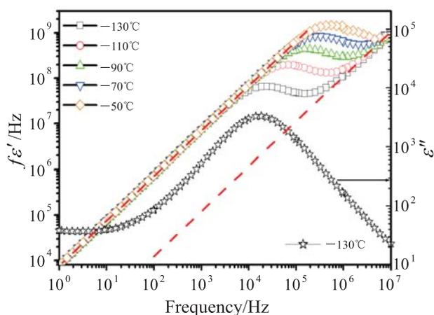
Fig. 3. Plot of  $f\epsilon'$  against  $f$  for CCTO at a number of temperatures (left and bottom axes) and frequency dependence of the imaginary dielectric permittivity at  $-130^\circ\text{C}$  (right and bottom axes)
