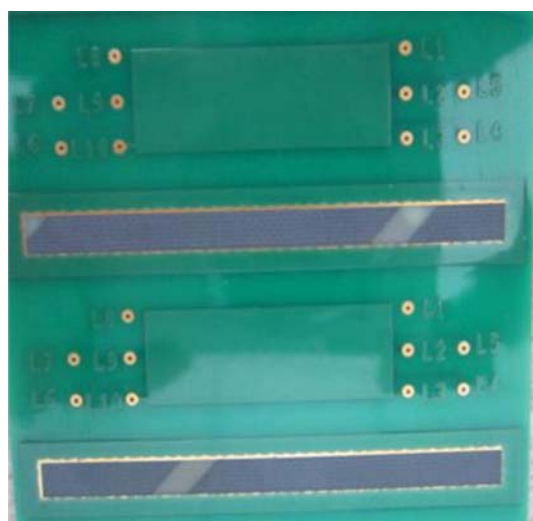
(a) rectangle capacitor embedded in 10-layer PCB
