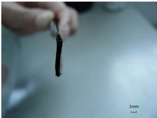
(a) 1\text{ mm} \times 1\text{ cm} \times 1\text{ cm} 悬浮碳纳米管阵列
