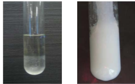
(a) saturated solution without additives (b) saturated solution with silica gel
