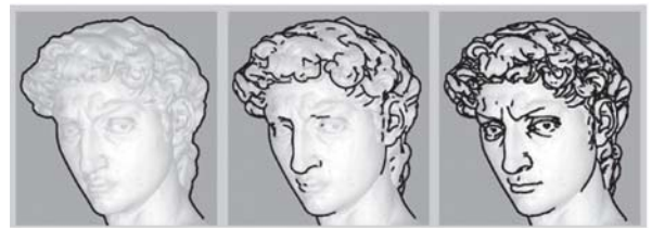
图 4 侧影(左)、轮廓线(中)及轮廓线+启发式轮廓线(右) Fig. 4 A sample of the rendered silhouette (left), occluding contours (center), and the integration of occluding contours with suggestive contours (right)
